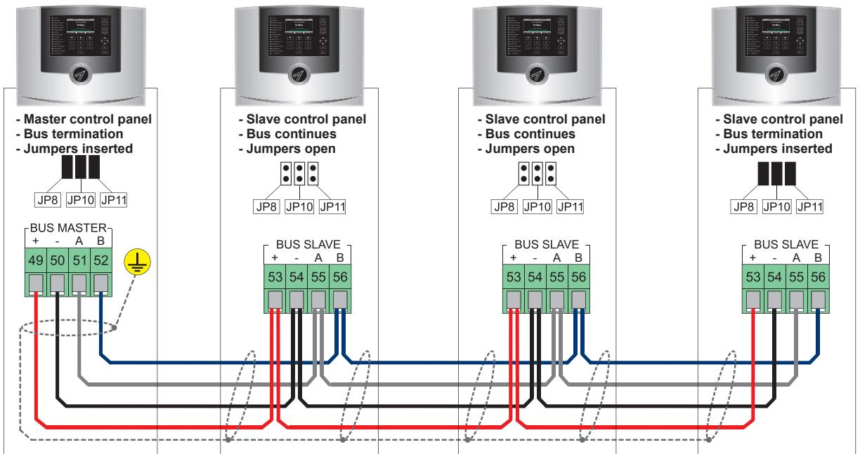
Closed loop connection to Master control panel
