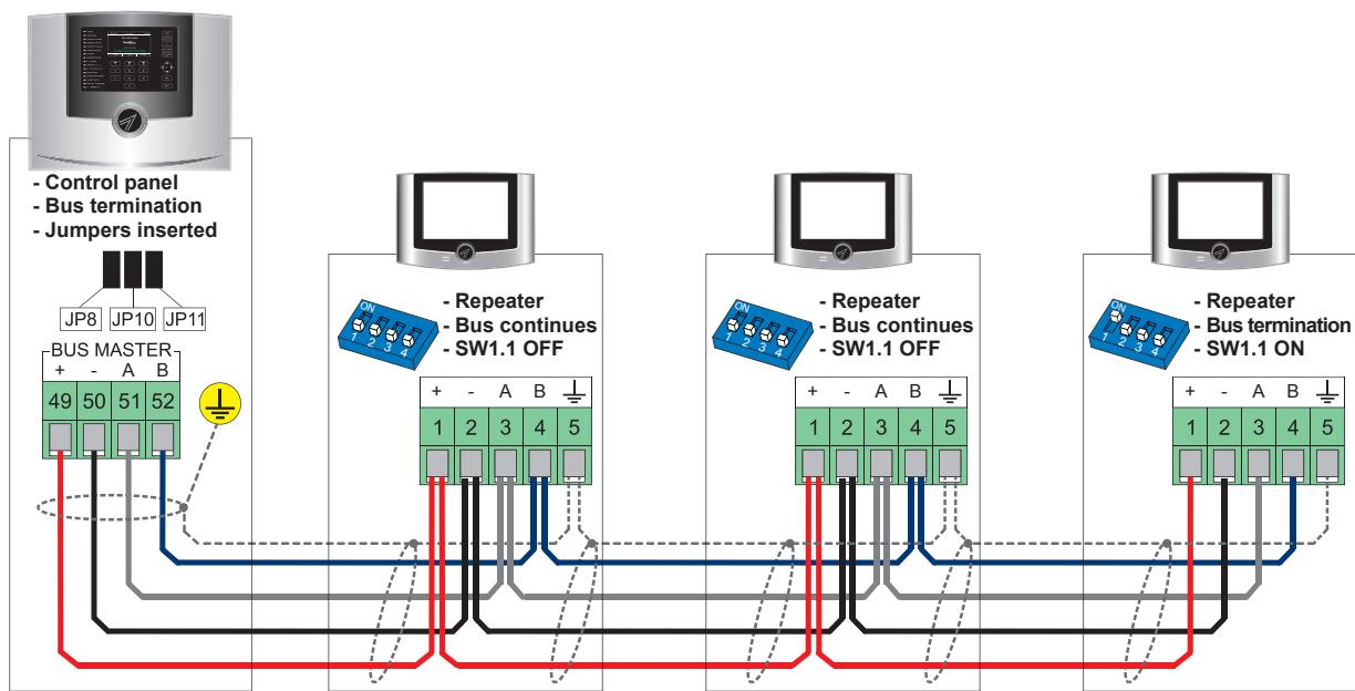
Open loop connection to Master control panel
