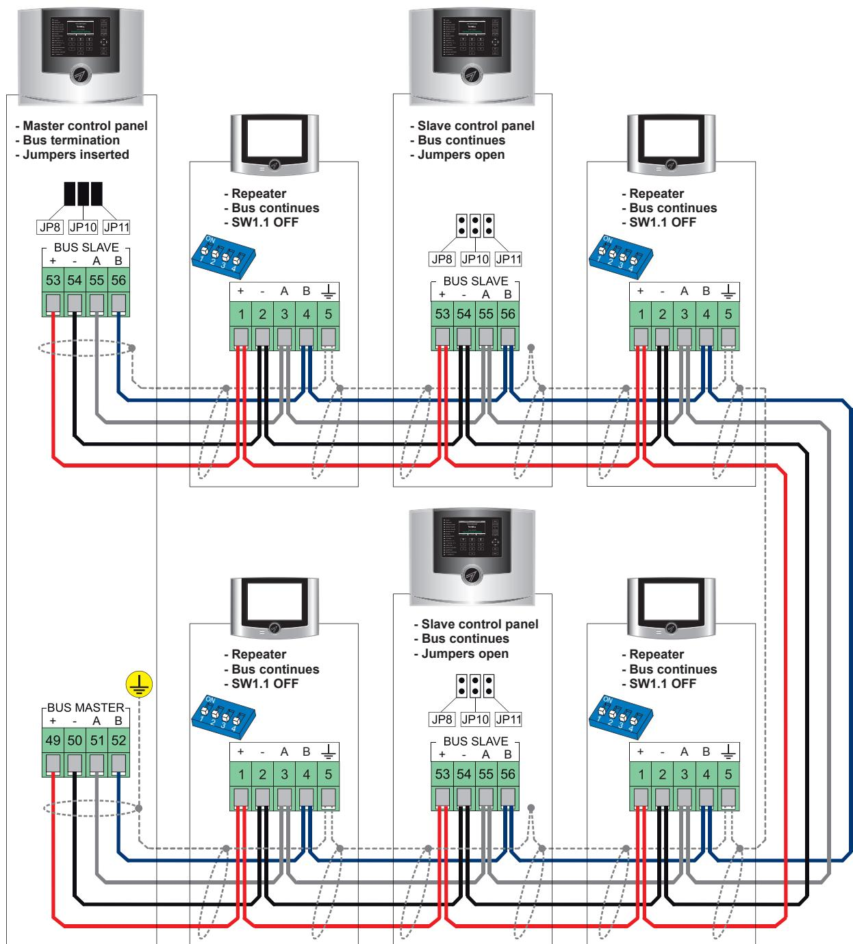
Connection of repeaters in open loop to Master control panel with fiber optic converter.
