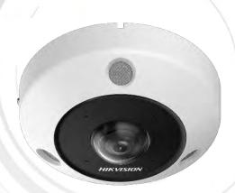
DS-2CD63C5G1-IVS is a fisheye network camera capable of providing a 360-degree panoramic image of its scene. The progressive scan CMOS sensor provides high-resolution images of up to 3504 × 3504. Up to 20 live view display modes, designed for 3 mount types, meet various user preferences. Three independently controlled IR lights offer a range of 15 m and provide good vision in low or even zero-light environment.
