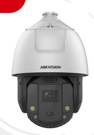
Hikvision DS-2DE7S425MW-AEB(F1)(S5) 4 MP 25× Network Speed Dome adopts a 1/1.8" progressive scan CMOS chip and a 1/2.8" progressive scan CMOS chip. With the 25× optical zoom lens, the camera offers more details over expansive areas.
