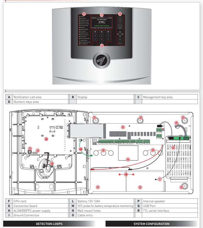
Each detection loop can manage 199 sensors and 99 modules. The programming of the devices connected on the LOOP is facilitated by the self-learning function. Device polling speed with full load Loop of less than 1 sec. For privileged devices, it is possible to set a higher frequency.
