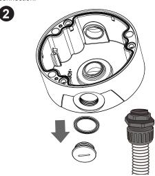
Install the cable gland and pass cables through it.
