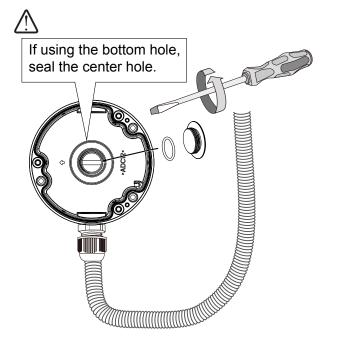
Make sure the rubber seal is properly installed to the center hole. The outer rim of the seal must be through and cover the
