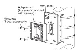
c) About mounting the camera onto adapter box (accessory provided with camera), please refer to
