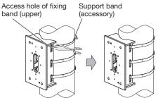
(5) For the remaining part of fixing bands, leave approximate 70 mm in the part of fixing band lock screw and use a tool (locally procured) to cut off the remaining part. Please treat the cut-off part to prevent injury.
